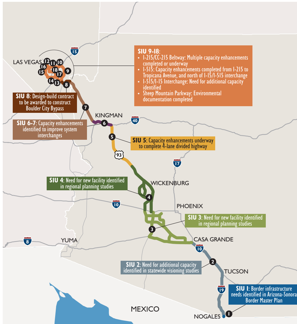
Figure 17 Illustrates the corridor’s 18 segments of independent utility (SIU), which are colored to clearly illustrate SIU endpoints. The status of project development activities completed to date are noted for each SIU. This segmentation does not include the Northern Nevada Future Connectivity Corridor segment, which requires additional study to determine logical corridor connections.
